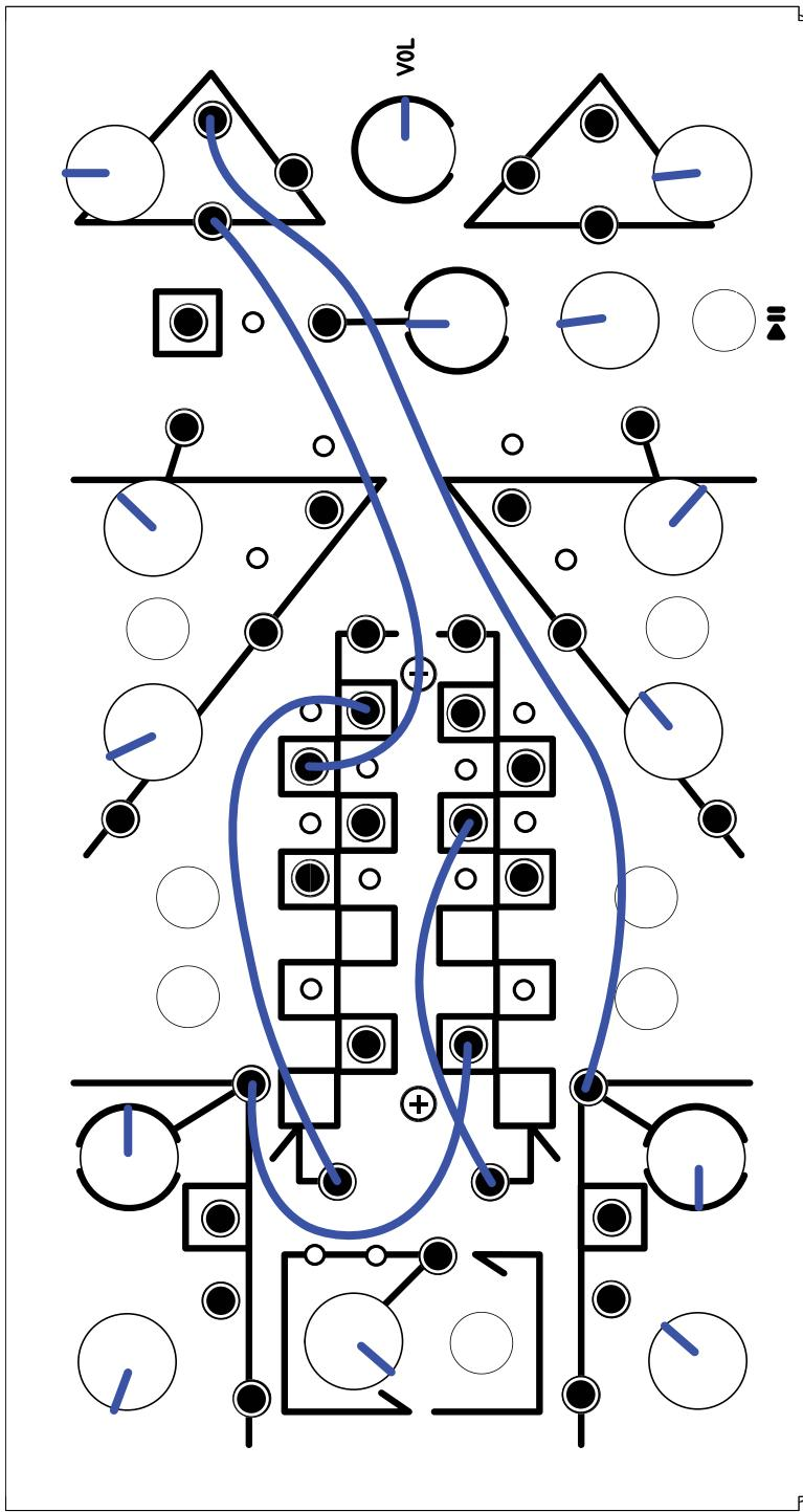
**“Rungler” Patch** How to implement a Rungler, a concept coined by Rob Hordijk. The Double Knot provides a good environment for experimenting with this fun and puzzling technique. Try it!
