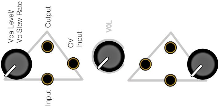
These two circuits are the only parts of the Double Knot which are not pre-wired to any other part of the system. These are independent signal processors with one knob two inputs and one output. Signal input is on the left, CV input is in the middle, and output is on the right. The knob sets the slew rate from nearly halted (full CCW) to pretty fast (full CW). When set as a VCA the level goes from off to roughly unity gain.
