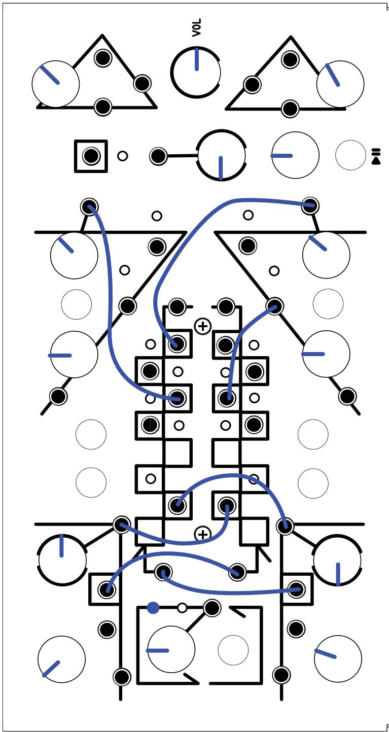
**Phasing Patterns** The registers here are looping data from the bit outputs back to the data input.
